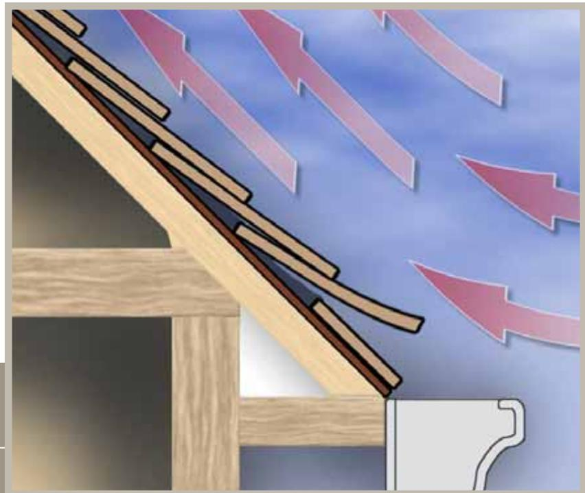
**Without the first layer being adhered at the edge properly, a strong gust of wind may lift the first layer of shingles and push them back up the roof, potentially taking other layers with it.**
