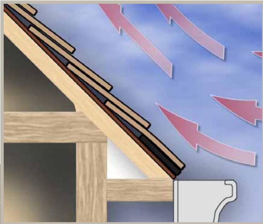
Using a starter shingle can help protect your home against wind uplift and water damage.
