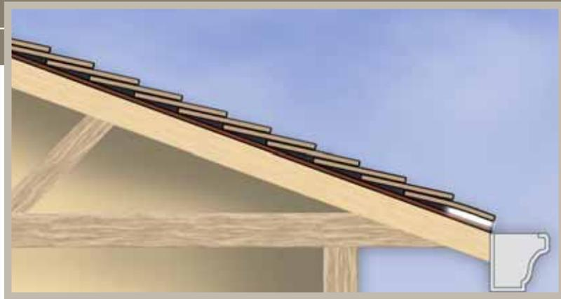
**The first course of a roof is one of the most important and often overlooked parts of the total system. According to an article on [roofingcontractor.com](http://roofingcontractor.com), leaving out the starter course is one of the most common mistakes in shingle application.**
