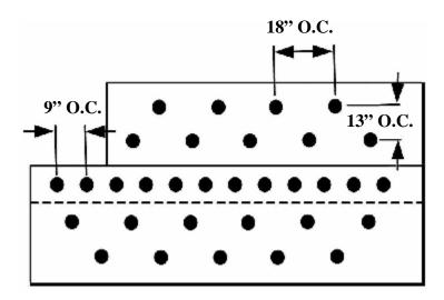
This attachment pattern applies to all 1 meter (39.4") wide Firestone APP compatible base sheets and cap sheets used as base sheets.
