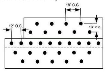
The attachment pattern below applies to all 1 meter wide (39.4") Firestone APP compatible base sheets and cap sheets used as base sheets. The Firestone MB Base sheet must be mechanically attached 18" (457.2 mm) o.c. in the side and end laps and 36" (914.4 mm) o.c. in two staggered rows in the field of the sheet. Each row shall be 12" (304.8 mm) in from the sides of the base sheet. See diagram below.
