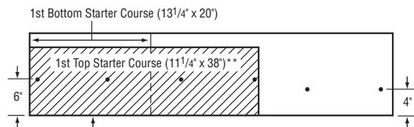
Extend the shingles over the rake and eaves about ½" (13 mm) if drip edge is used, or about ¾" (19 mm) if no drip edge is used. \*\*Continue along eave with 11¼" x 40" Top Starter Course shingles, butted against the in-place Top Starter Shingles and Flush to the Lower Edge of the Bottom Starter.
