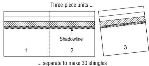
Figure 15-19: Separate to make 3 cap shingles.
